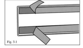
**STOP NOTE:** Once the release liner is removed from the molding, the surface of the foam tape must not be touched!
